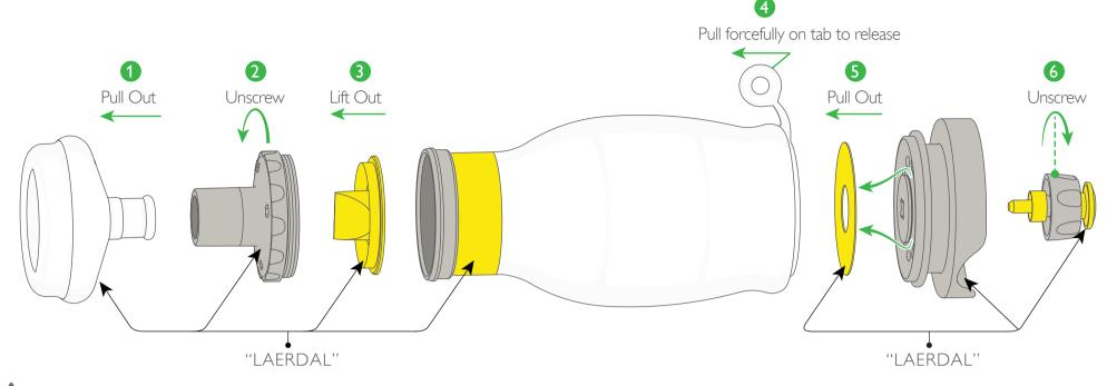
Do not disassemble parts beyond the steps shown. For proper function, make sure to only use parts marked LAERDAL (locations as shown above).
