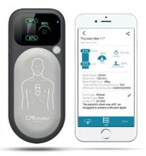
The CPRmeter 2 device with QCPR technology provides real-time coaching and summative feedback to help rescuers optimize CPR performance in a clinical setting. Combined with the new free CPRmeter app, organizations can now drive quality improvement initiatives with detailed and sharable insights on CPR performance.
